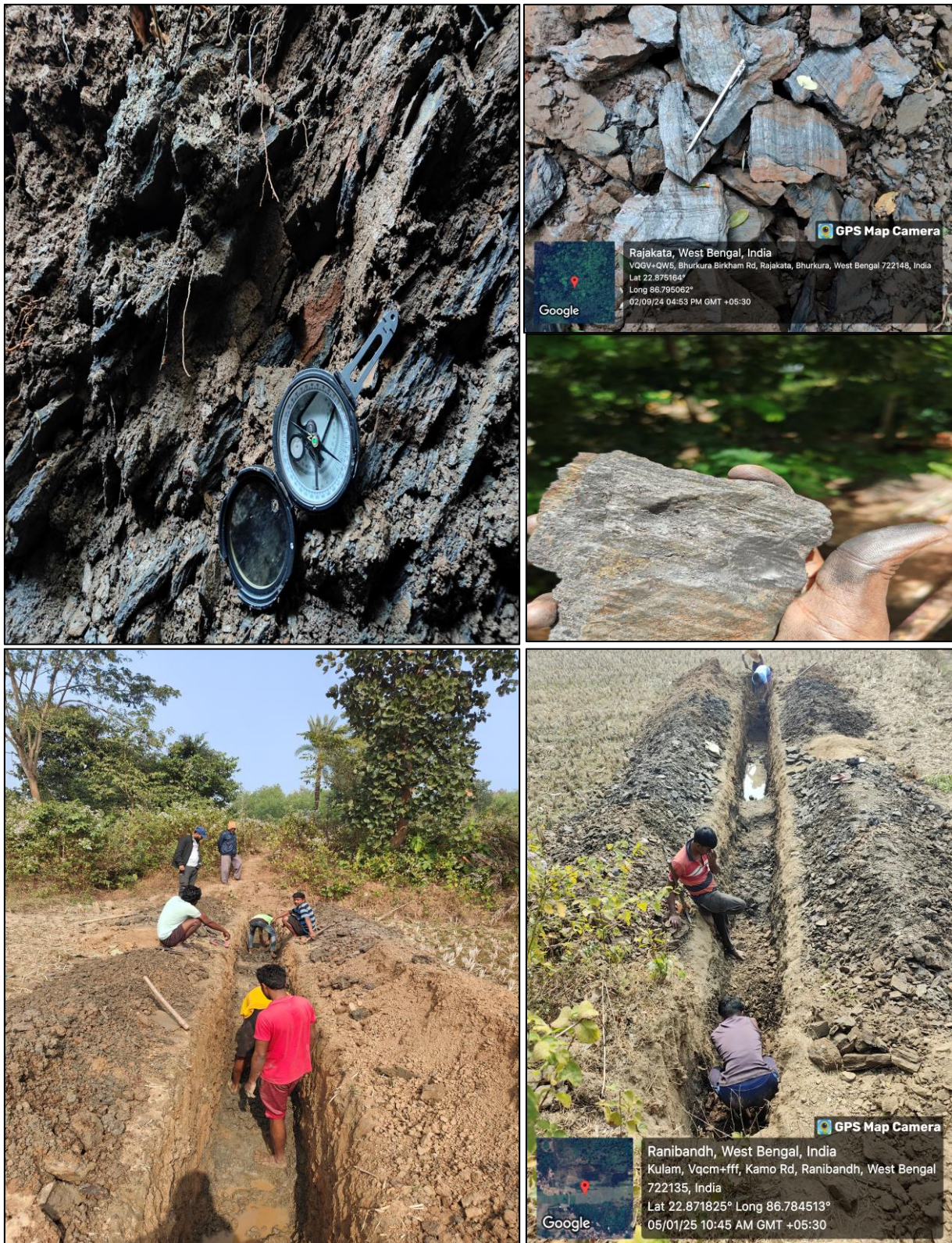
Fig.6.19 Field Photographs showing trenching activities and in-situ graphite bands exposed during trenching.
