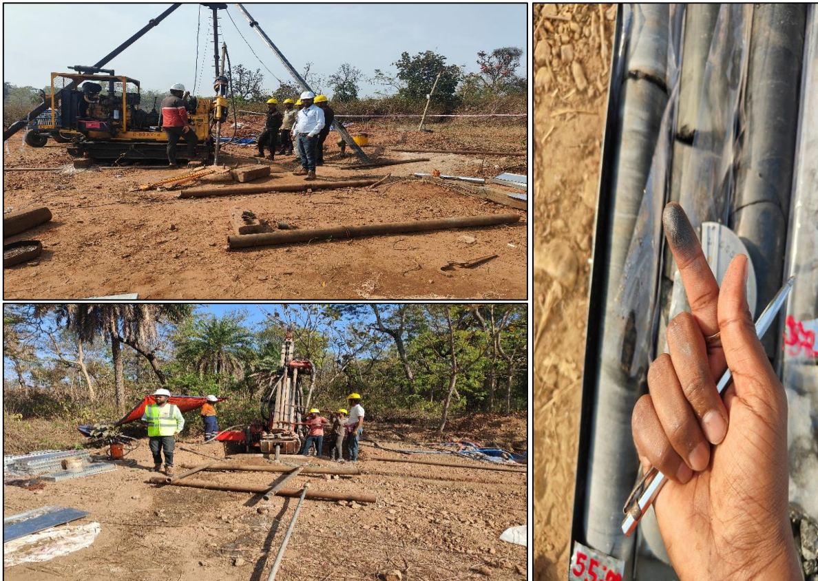
Fig. 9.1 Field photographs showing the drill site and the deployed drill rig in operation during exploratory drilling at Ranibandh Block.
