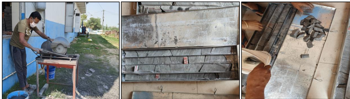
Fig.9.11 Photographs showing stages of core samples cutting.
