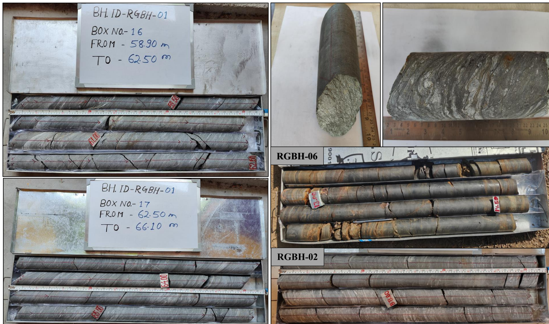
Fig. 9.3 Core photographs of various boreholes showing graphite bearing quartz mica schist.
