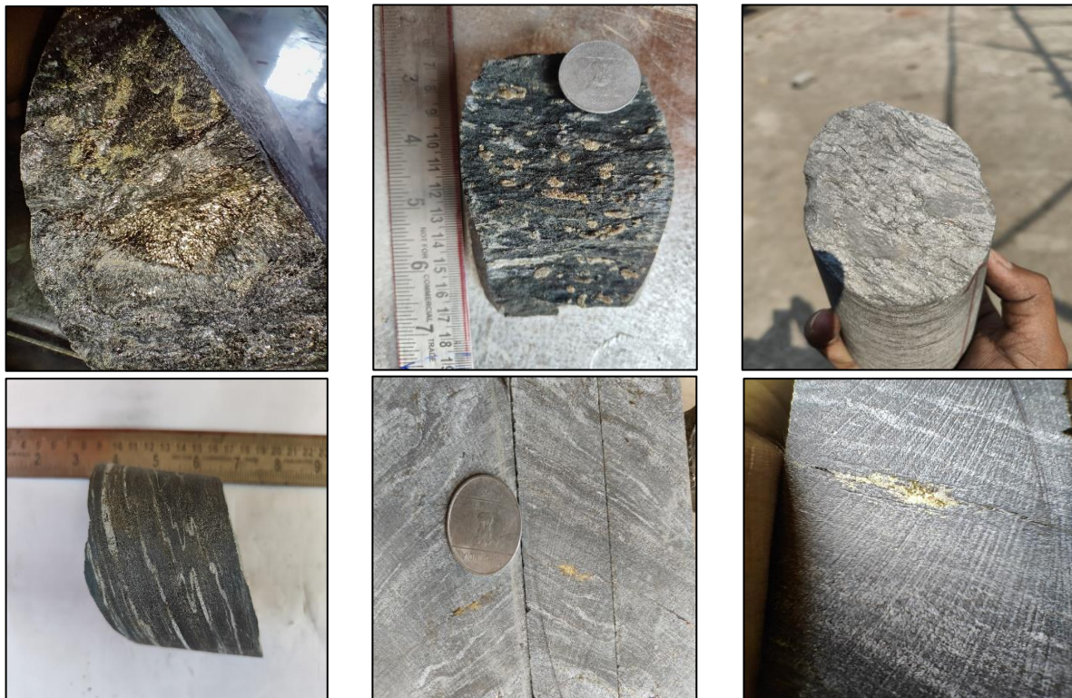
Fig. 9.2 Showing Core photographs of graphite schist with interlayered cenululated quartz veins with emplacements of sulphides (Pyrite, chalcopyrite etc.) as specks, streaks and stringers.
